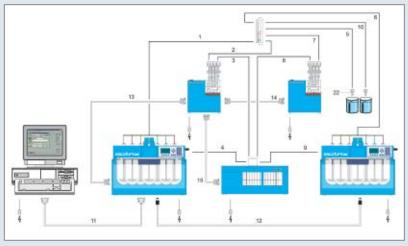
SOTAX AT 7smart double off-line automated system for dissolution test according to USP with solvent replacement
